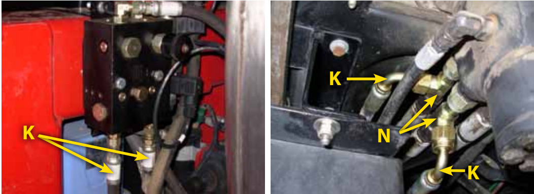
Figure 1-7: Install the Steering Hoses and Adapters
