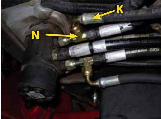
Figure 1-8: Install The Tank Hose
