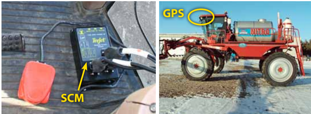
Figure 1-13: Recommended Electronics Installation
