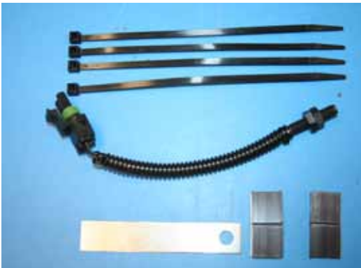
Figure 1-11: Install Steering Disengage Switch (Kit 91-07011)
