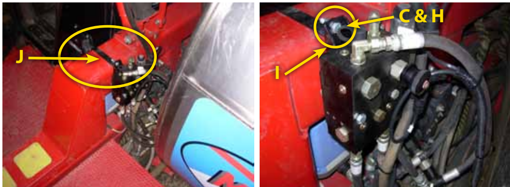
Figure 1-5: Install Mounting Bracket for FieldPilot Valve
