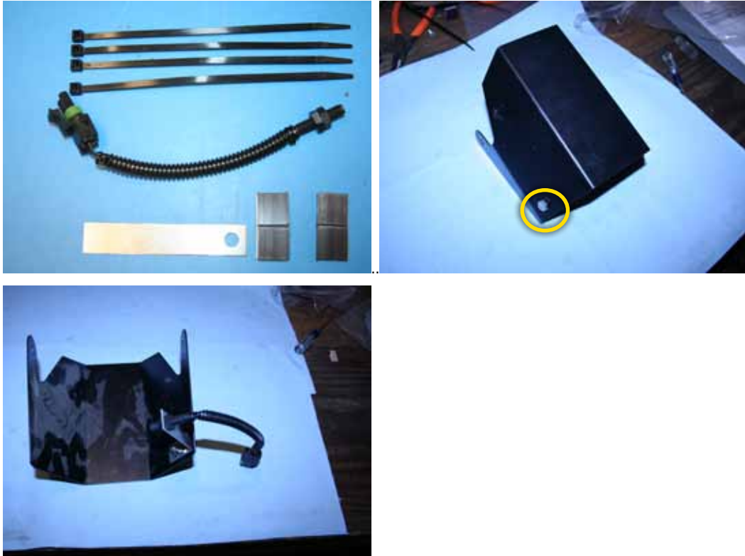
Figure 1-11: Installing the Steering Disengage Sensor
