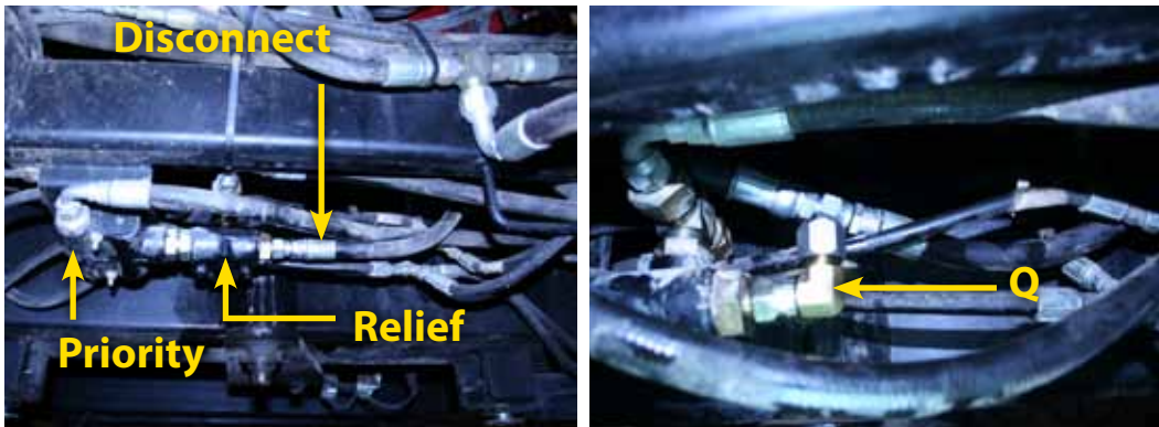
Figure 1-9: Installing the EF Fittings and Hose
