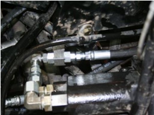
Figure 1-10: Install the Shuttle Tees
