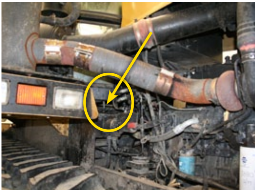
Figure 1-4: Install Mounting Bracket for FieldPilot Valve
