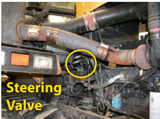
Figure 1-9: Prepare the Steering Ports On the Steering Valve
