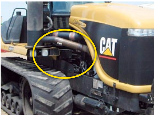
Figure 1-5: Install Mounting Bracket for FieldPilot Valve
