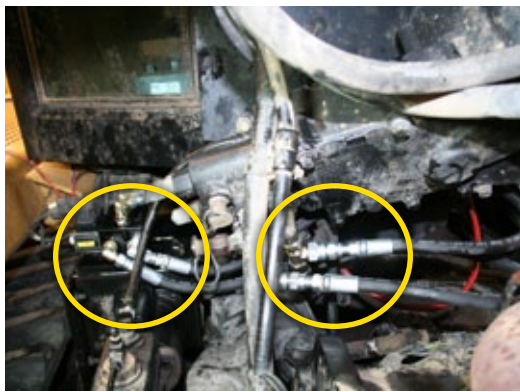
Figure 1-13: Install the Pressure and Tank Hoses
