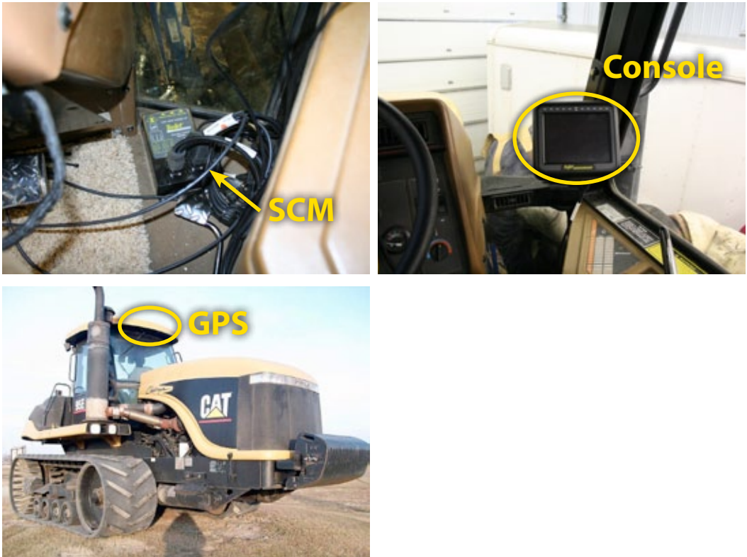
Figure 1-17: Recommended Electronics Installation
