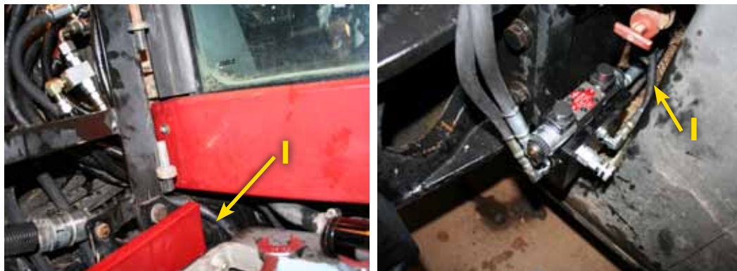
Figure 1-6: Install Steering Output Hoses
