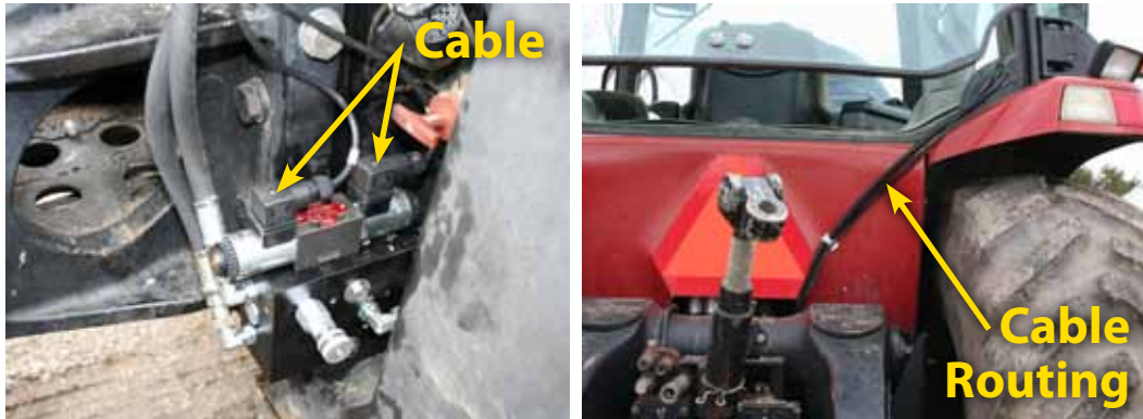
Figure 1-12: Install the Valve Control Cable
