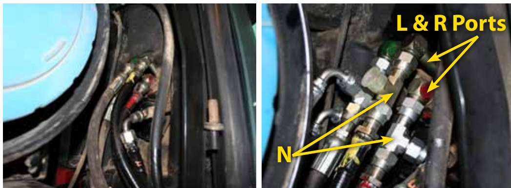
Figure 1-5: Install Steering Output Adapters
