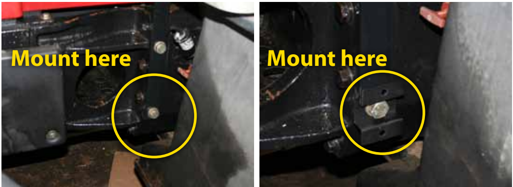
Figure 1-3: Install Mounting Bracket for FieldPilot Valve
