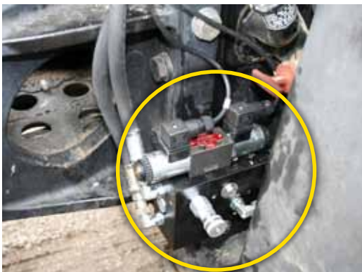
Figure 1-4: Mount the FieldPilot Valve
