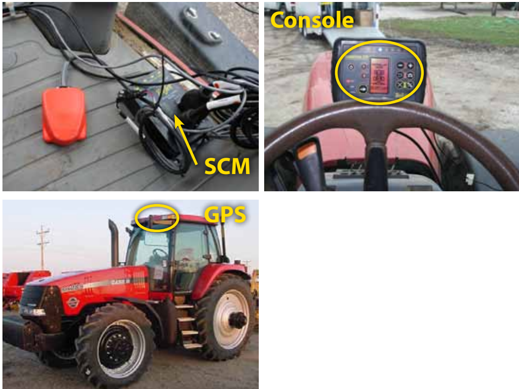
Figure 1-15: Recommended Electronics Installation
