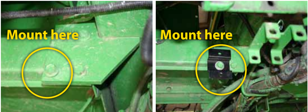
Figure 1-3: Mount the FieldPilot Valve Bracket
