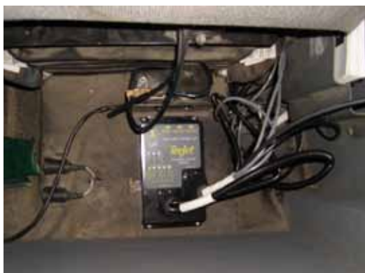
Figure 1-11: Recommended Electronics Installation
